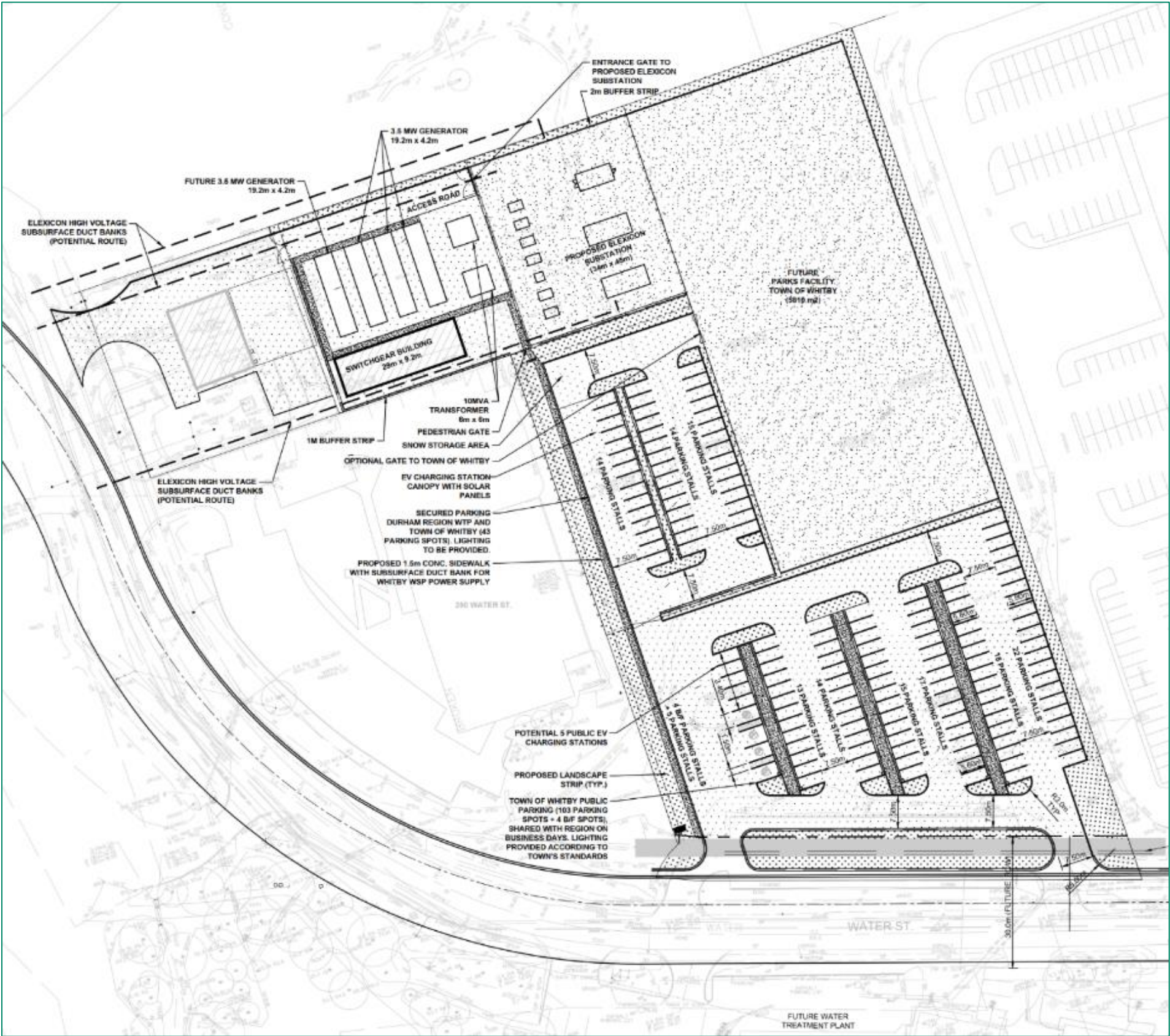
Figure 3-5: Ultimate Site Plan for 270 Water Street
